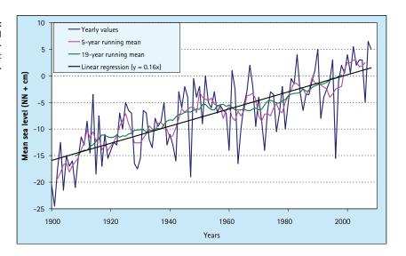
tide, it is important that human impacts are duly considered. For example, embankments or corrections to navigation channels can significantly influence tidal dynamics and MSL.
