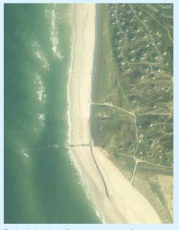
Fig b.: Aerial view of the southern part of the tetrapod construction on Sylt in 2005 (Note that the section north of the groin is hidden under primary dunes)
