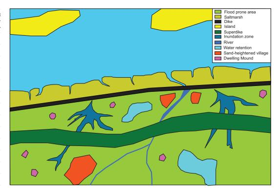
Figure 12: Schematic overview of typical coastal zone elements.
