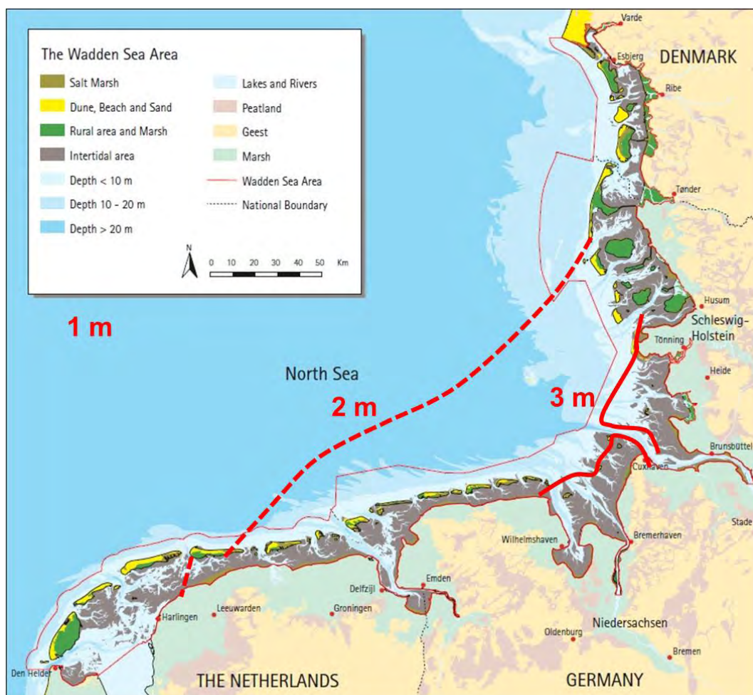
Figure 9.3.1: Overview of tidal range of the Wadden Sea area; comparing figure 3.2.3 with this figure indicates that ebb-tidal deltas near the 3 m tidal range are at the upper limits of the zone where they can exist.
